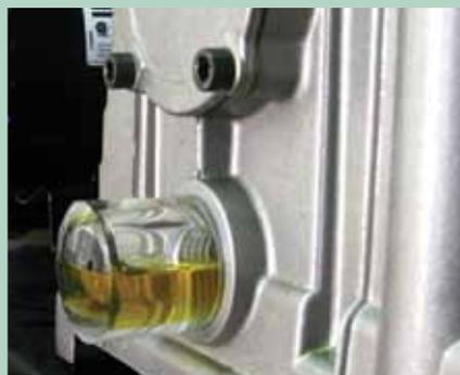
With Esco's 3-D BullsEye™, the reservoir oil can be inspected easily and accurately.
