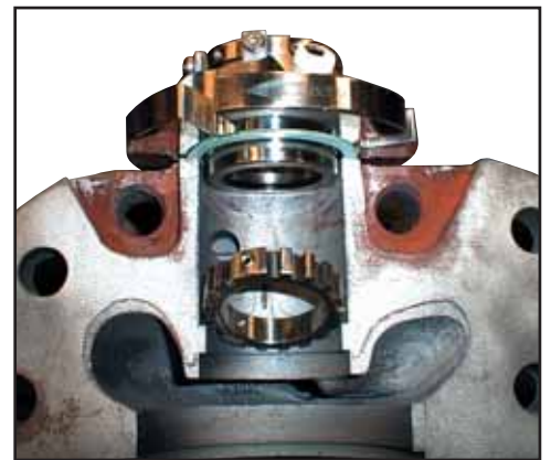
Separate conventional seal and pumping ring configuration.
