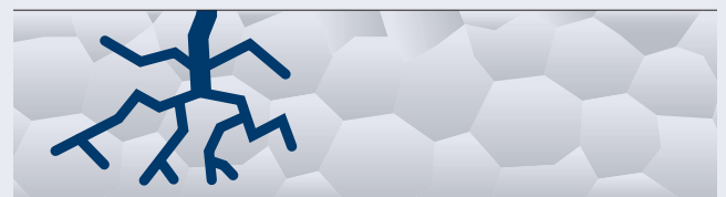
Fig. 1.6.10: Stress corrosion cracking
