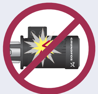
Fig 1.4.6: With non-sparking motors ExnA, no ignition is likely to occur.
