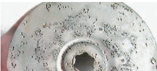
Pitting corrosion of EN 1.4401 (AISI 316)
