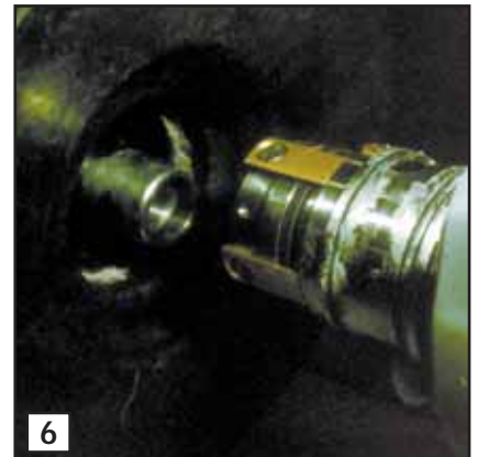
6 Ensure the anti-rotation lugs on the seal are aligned at 12 o'clock and 6 o'clock and the inlet port on the seal gland is at 6 o'clock, then slide the seal onto the pump shaft.
