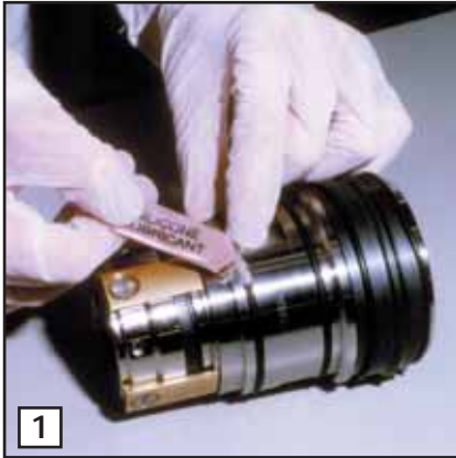
1 Lightly apply grease to the bare shaft and seal gland elastomers.
