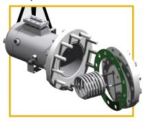
Unscrew the bolts and remove the bottom flange. This gives full access for cleaning.
